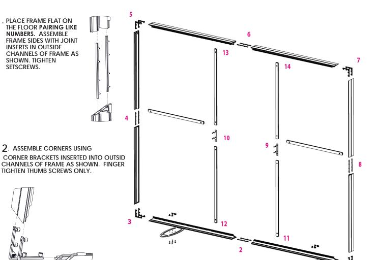
3. ASSEMBLE LONG VERTICAL SUPPORTS BY COUPLING THE 2 SECTIONS USING THE VERTICAL INSERT AND INCLUDED HARDWARF.
