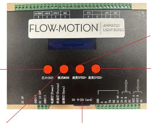
Increase the speed of the program by pressing the "Speed+" button.
