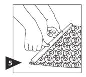
Apply even pressure to the snap-lock profile to lock graphic into place.
