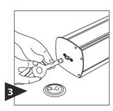
Holding tool firmly, twist clock-wise to re-tension. Wind 33 full turns. Return pin back to lock position. Replace cover.
