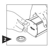
Guide the slot of Re-Tension Tool over the exposed metal pin. Move pin from lock position into center circle. The pin can now turn for re-tensioning.
