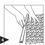
Once the snap-lock profile is open, insert top portion of graphic into profile.
