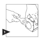
Face back of unit with the pole slot closest to you. Use the edge of the Re-Tension Tool to gently pop off the cover on the right side of unit.
