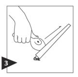
Use the edge of Re-Tension Tool to open the snap-lock profile.
