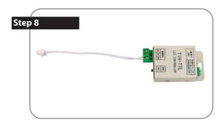
The provided light controller will have the animation preinstalled. Connect the light curtain connector as seen.
