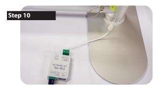
Connect the light curtain to the light controller. This connector will be found on the bottom right from the back of the display.
