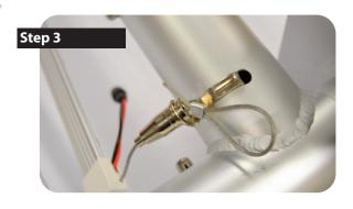
Hook the light curtain clips into the two holes located on the top of the connecting tubes. Proceed to then hook the light curtain clips into the two holes located at the bottom connecting tubes. Adjust the tension by pressing down on the clip, and pulling on the cable.
