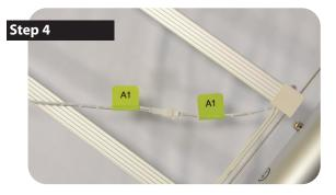
To connect the light curtains together. Find the connecting wires located on the back of the display. The connecting wire will run diagonally across the back, match the identifier with the corrosponding identifier.
