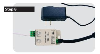
Attached the power supply to the light controller. An outlet is require to plug in and power the controller for the display.
