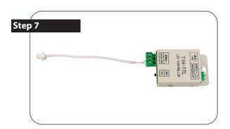
The provided light controller will have the animation preinstalled. Connect the light curtain connector as seen.
