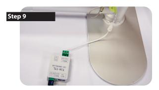
Connect the light curtain to the light controller. This connector will be found on the bottom right from the back of the display.
