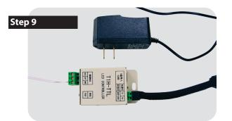
Attached the power supply to the light controller. An outlet is require to plug in and power the controller for the display.
