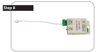
The provided light controller will have the animation preinstalled. Connect the light curtain connector as seen.
